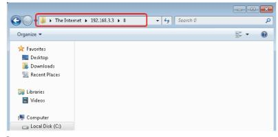
**2.** Copy the created user program "R12\_SampleProject.out" to the program memory '0' in the C Controller module by a drag and drop operation.
