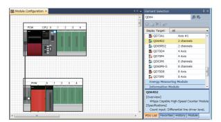
**1.** Create a module configuration in accordance with the actual configuration by dragging each MELSEC-Q series module from the Element Selection window and dropping it onto the Module Configuration Diagram.
