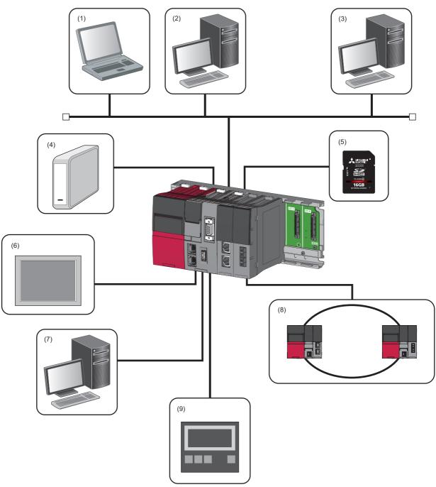
(1) Personal computer for maintenance (Telnet function and FTP function)
