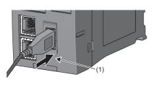
Connect a connector of USB Mass Storage Class-compliant device or USB cable to the USB connector (1). Firmly insert the connector to prevent it from falling out.
