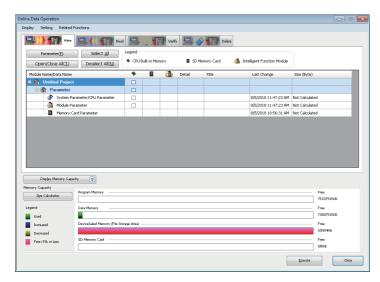
4. Select "System Parameter/CPU Parameter" and "Module Parameter", and click the [Execute] button.
