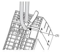
**3.** Pass the USB cable (3) through the fixing band to fix.
