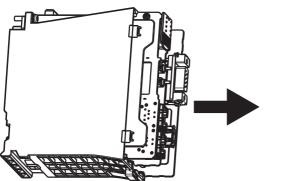
**2.** Remove the printed circuit board from the case.
