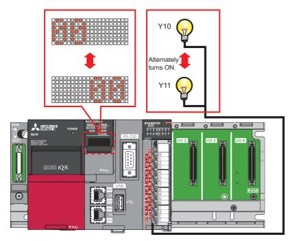
**3.** To check the operations again, reset the C Controller module.
