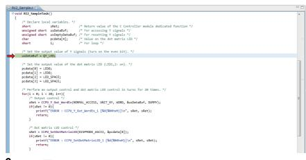
**9.** Click  $\underline{\circ}$  in the "Debug" window to debug a program by one step.
