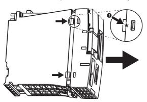
Lift the ⑦ (★) portion on the side of the C Controller module, and remove the front cover.
